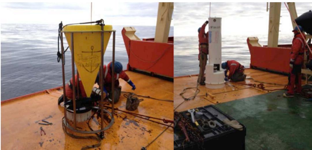
*Figure 3. Pictures of both sediment traps before being redeployed again to sample until next years cruise.*
