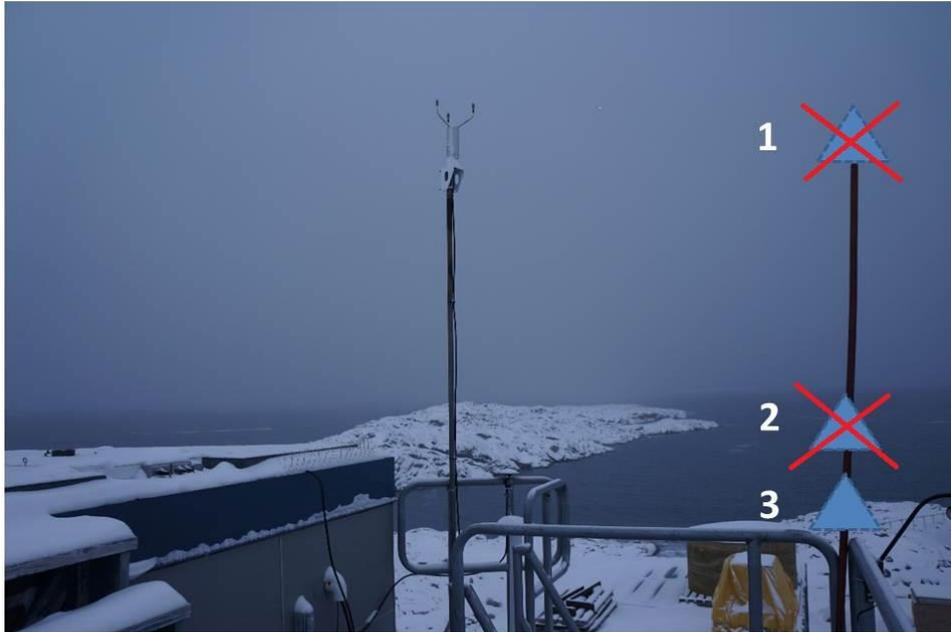
**Figure 1.** Westward view from the roof of the Terra Lab building. Proposed positions #1 and #2 were not approved, and the antenna was installed at position #3.
