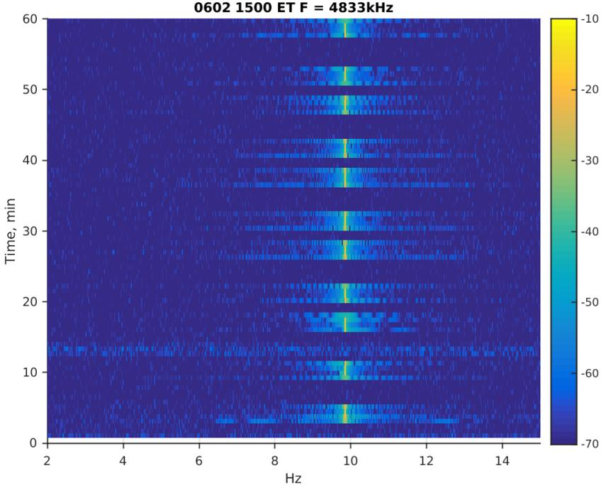
**Figure 4.** An example of Vernadsky-Palmer sounding on June 2, 2015 made at three interlaced frequencies. One of the three sounding frequencies is shown in this plot. Each frequency takes 2 min of operation.
