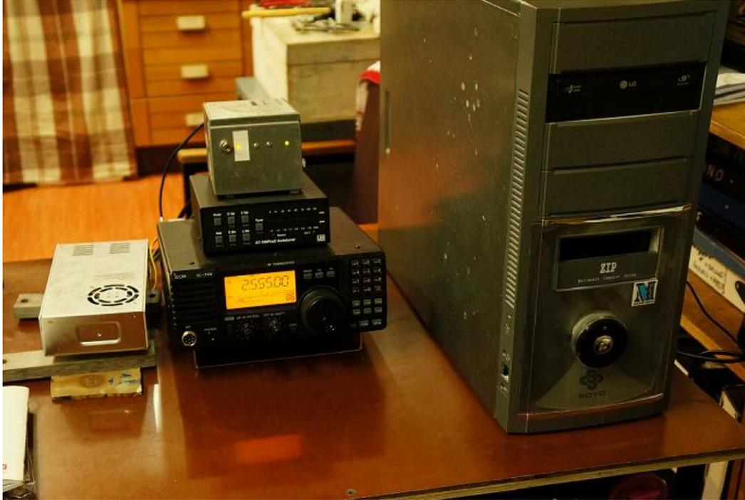
**Figure 3.** Transmitter assembly at Vernadsky Station. The system includes ICOM-718 transceiver, antenna tuner, power supply box, modulator, and PC computer.
