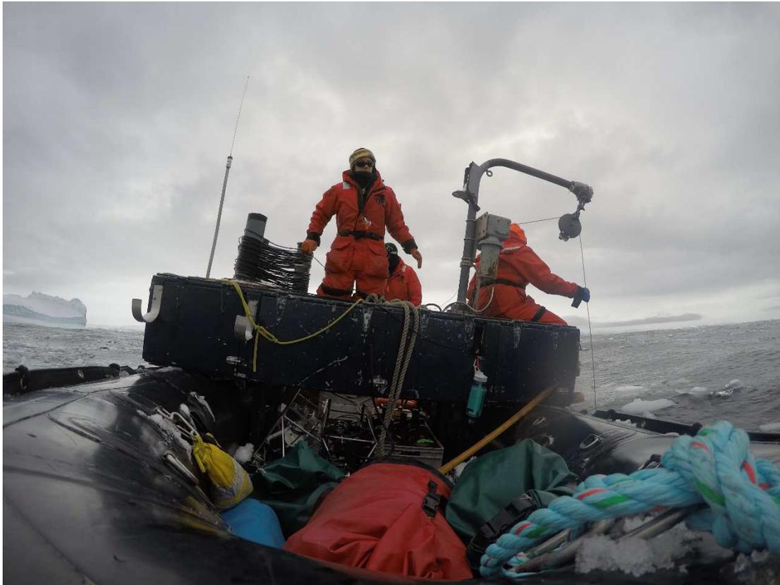
**Image 1.** From left to right: Rachel Kaplan, Conor Sullivan, and Naomi Shelton sample at Station E on February 26, 2015. The winch is used to lower Go-Flo bottles into the water for collection at discrete depths, with the deepest sample at 65 meters.
