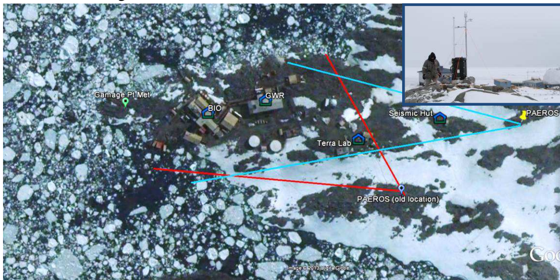
Figure 2: PAEROS sites for aerosol observations at Palmer Station. BIO and GWR mark the location of the main local sources of aerosol. Red and blue line mark wind sectors when expect to sample air from the station. The inset image shows PAEROS on the ridge above the station.
