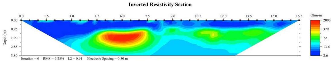
**Figure 4:** One resistivity image collected near low tide on 1/17/31. Offshore is to the left. The far right side represents the high high tide line. The cool colors are saltier water and the warm colors are fresher water. At this time period, the last 6 meters of the cable (left side of image) is submerged.
