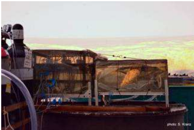
Figure 6: Experimental setup to acclimate phytoplankton to different CO 2 concentrations. The gas-cylinders are connected to the incubation bottles filled with seawater. The screening blocks roughly 50-60% of sunlight mimicking a water depth of 5-10m.
