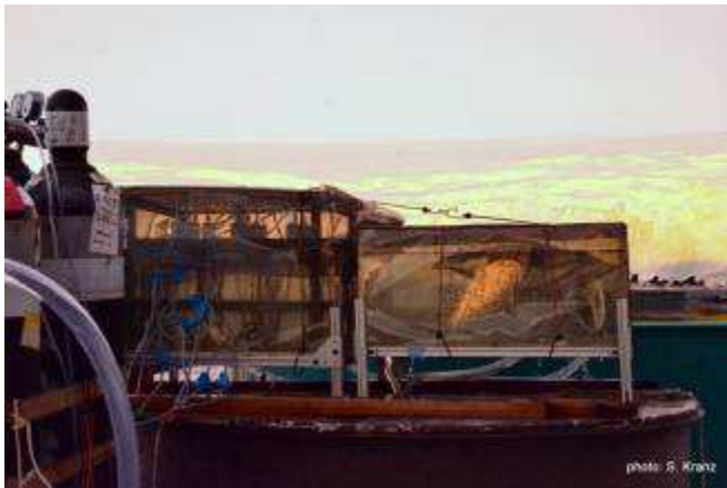
Figure 4: Experimental setup to acclimate phytoplankton to different CO 2 concentrations. The gas-cylinders are connected to the incubation bottles filled with seawater. The screening blocks roughly 50-60% of sunlight mimicking a water depth of 5-10m.
