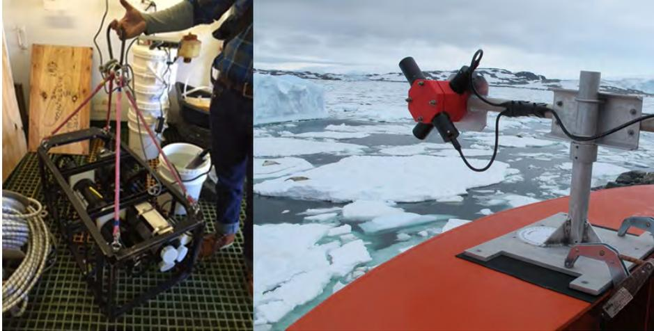
**Figure 3.** Optical cage (left) and shipborne radiometer (right)
