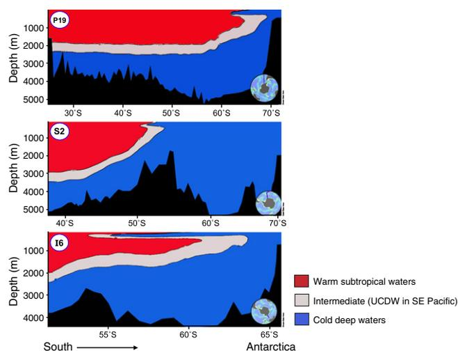
**Fig. 3.** 3-color WOCE temperature sections along the tracks crossing the ACC in polar projection (in Fig. 2) labeled same as those sections. Sections show that tilt of the isopycnals associated with ACC prevent warm tropical waters (red) from reaching Antarctic continental margin. Warm UCDW layer (white) slips along the tilted isopycnals to reach the continental slope in section P19 along the WAP, and elsewhere only reaches the northern limit of the polar waters.
