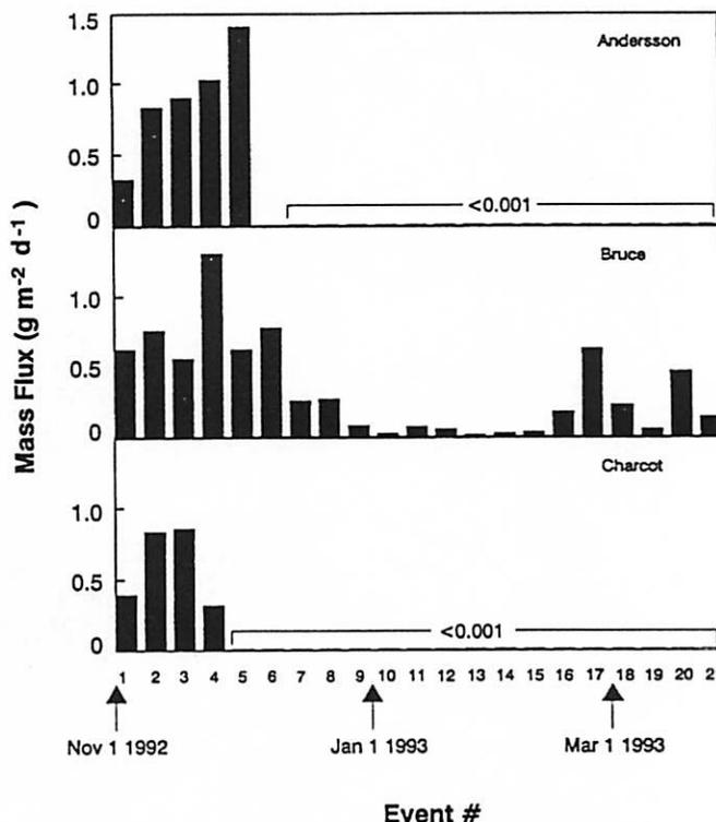
Figure 2. Time-series of mass fluxes (expressed in milligrams of total mass per square meter per day) for three sediment trap moorings located near Hugo Island (see table for exact coordinates). Each event was equivalent to a collection period of 6.71 days.
